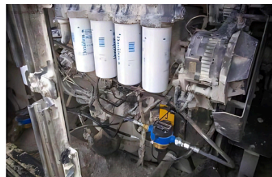
Mounting a pair of fuel flow meters on a mining excavator
