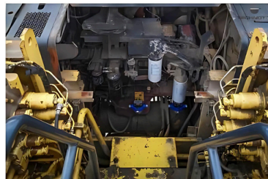
Fuel flow meters are installed in Komatsu fuel supply system Komatsu PC1800
